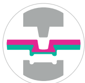
Clinching, TOX ® - Sheet metal joining
